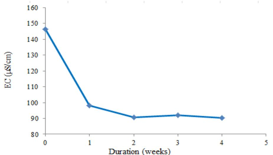
**Figure 6:** Effect of vermiremediation on soil contaminated with diesel engine oil's EC
