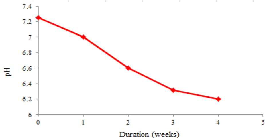
**Figure 5:** Effect of vermiremediation on soil contaminated with diesel engine oil's pH
